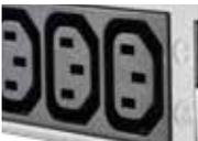
3 Outlet sockets for instrument or equipment (max 8 A)
